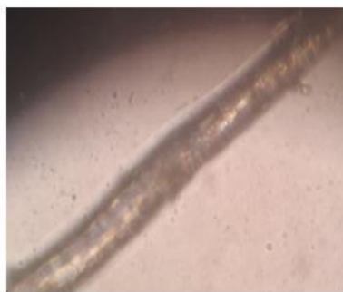
(C) Longitudinal view of Ramie Fibre
